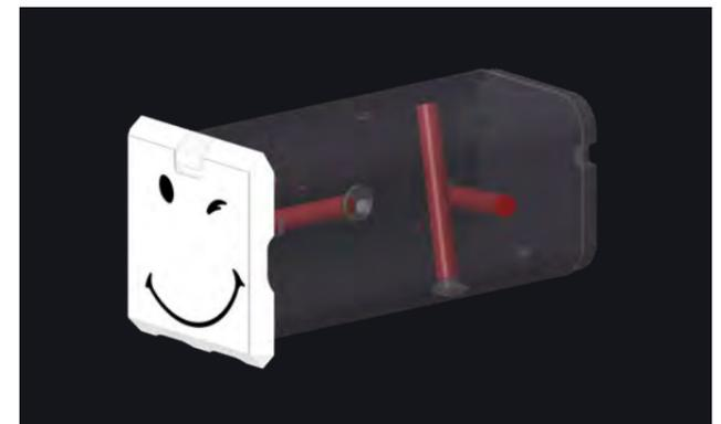
RUBY Insert "Alignment/Isocenter Check" for LINAC QA
